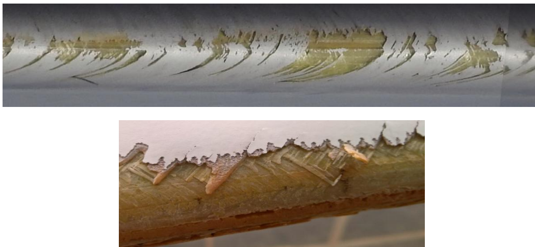
Figure 9: Examples of Severe (Category 5) Leading Edge Erosion
