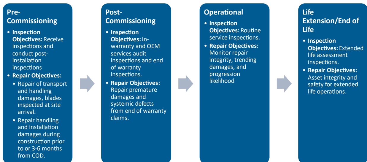
Figure 2: Wind farm/blade life cycle and where inspection and repairs typically are done
