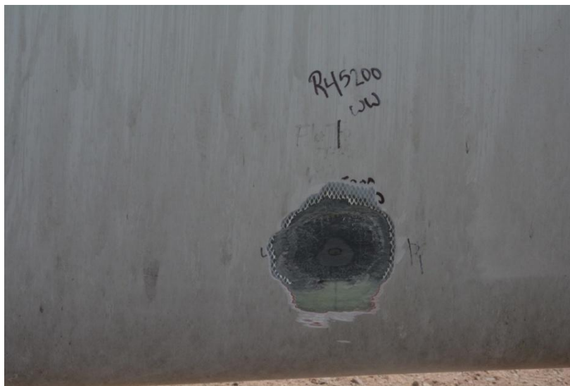
Figure 15: Illustration of a Grind to the Bottom of a Lightning Damage to a Carbon Spar Cap
