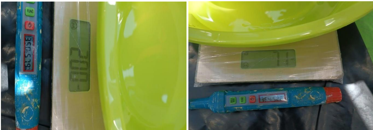
Figure 21: Documentation of Weighing Out the Resin and Hardener
