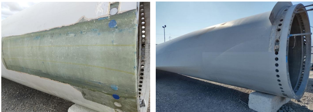
(a) Sanding of the Finished & Cured Laminate (b) After Paint and Drilling of Barrel Nut Holes
