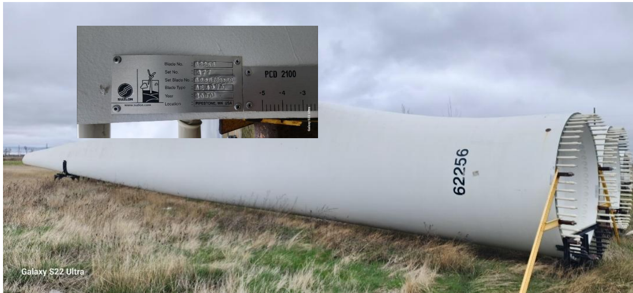
Figure 11: Example of Blade Serial Number Marking and Nameplate
