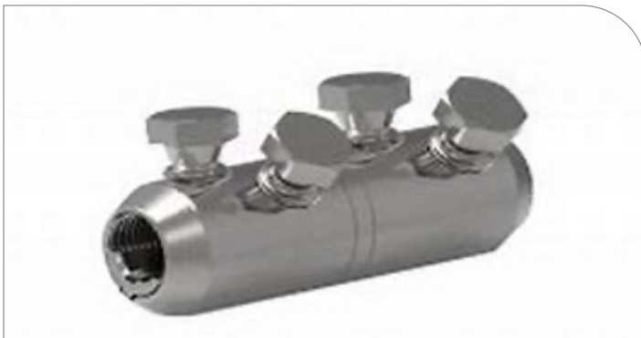
Figure 1 (left) One style of shear bolt coupling with hex head bolts, operated by a typical socket set. Fig 1 (Right) Another manufacturer's shear bolt coupling with Allen head bolts. Connectors would have a bolt connection pad on one end. With either type, the shaft of the bolt will shear when the proper torque is reached
