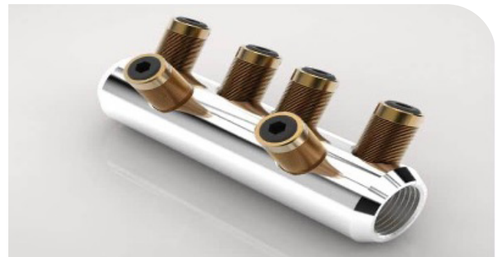
Figure 1 (left) One style of shear bolt coupling with hex head bolts, operated by a typical socket set. Fig 1 (Right) Another manufacturer's shear bolt coupling with Allen head bolts. Connectors would have a bolt connection pad on one end. With either type, the shaft of the bolt will shear when the proper torque is reached
