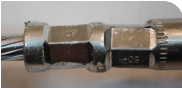
Figure 3 Example of a compression connector with a slight “banana” shape but, more importantly, showing a sharp tab left from the compression tools. This tab will become a point of Partial Discharge within the insulating body and can lead to failures.
