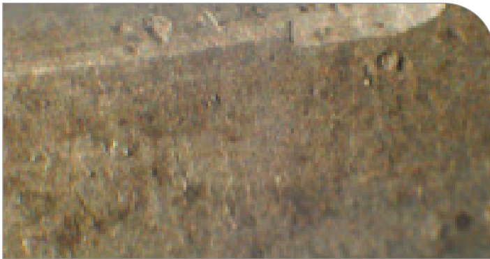
Figure 4 (left) Microscopic examination of a conductor sent to the laboratory for a Root Cause Analysis after a similar cable failed (and was destroyed) in service. Seen is one outer strand of a multi-strand cable, with no evidence of wire brushing, nor of antioxidant. Figure 3 (right) Microscopic examination of an example of a single strand of a similar sized multi-strand wire after wire brushing and application of antioxidant. (Photographs courtesy of Imcorp).
