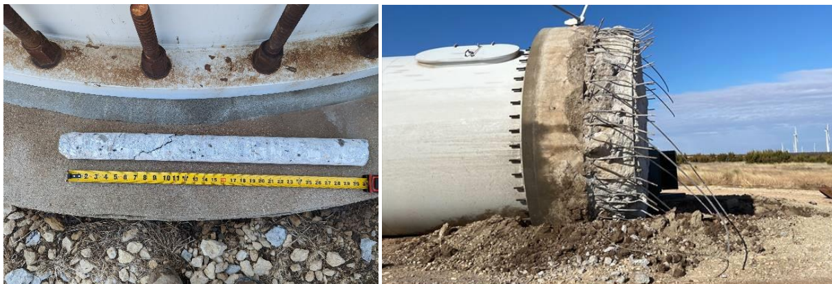
Figure 2019. Cracked concrete core taken at the anchorage pullout area in the left photo, turbine collapse due to foundation overloading event and anchorage pullout failure in the right photo.
