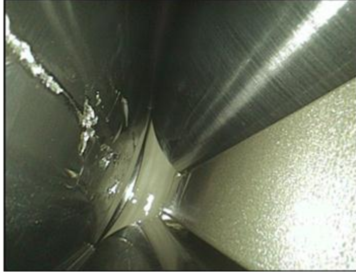
Figure A. Example of damage to the inner race of a high speed bearing documented with a borescope.
