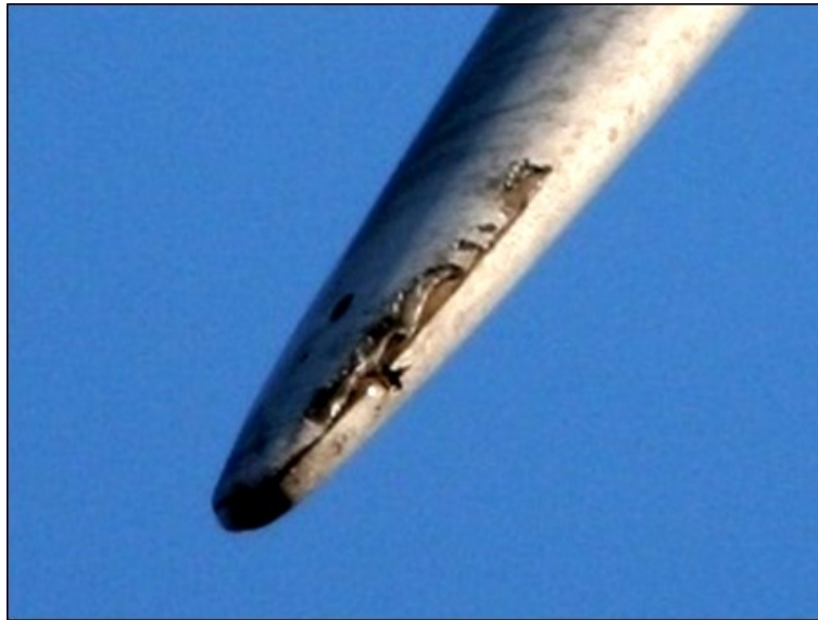
Example of blade damage documented with ground-based digital photography.
