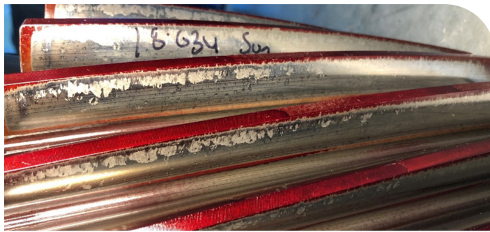
Figure 8: Micro pitting along addenda of gear teeth
