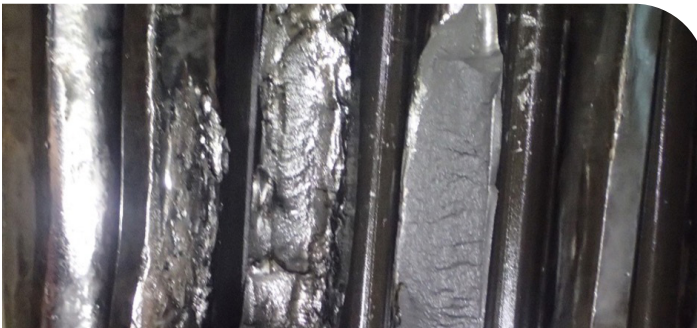
Figure 15: Completely brittle fracture on the tooth to the far right, causing mixed mode fracture of the tooth behind it. Total brittle fractures due to one load cycle are also known as tooth shear.
