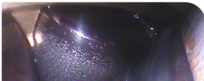
Figure 22: Bearing roller that was found to have micro pitting
