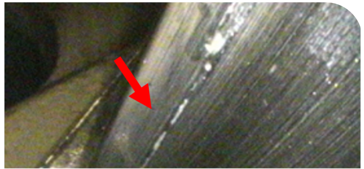
Figure 31: Straight-line micro pitting
