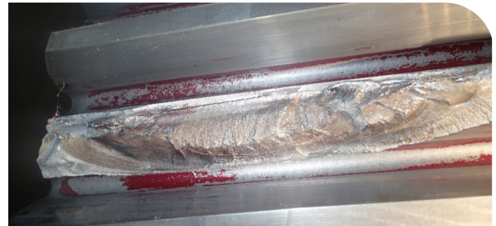
Figure 16: Mixed mode. Mostly brittle fracture shown, as the tooth was overloaded almost to the point of fracture, then the crack propagated in a ductile fashion during subsequent loads until liberation.
