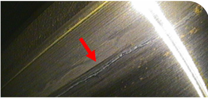
Figure 30: Scratch on gear tooth
