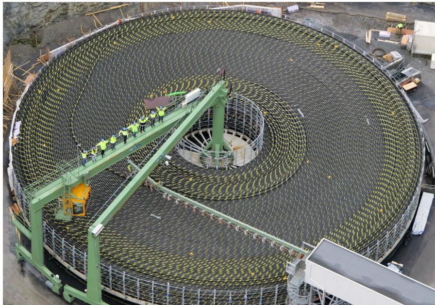
Picture: Turntable used for storage in a HV submarine cable factory
